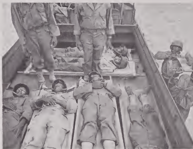
FIGURE 10. Demonstration of casualty evacuation by DUKW during demonstration for Surgeon General, POA, on Oahu. Bottom layer of six litters is complete, first litter of top layer is about to be passed up. Space is left for two attendants.
